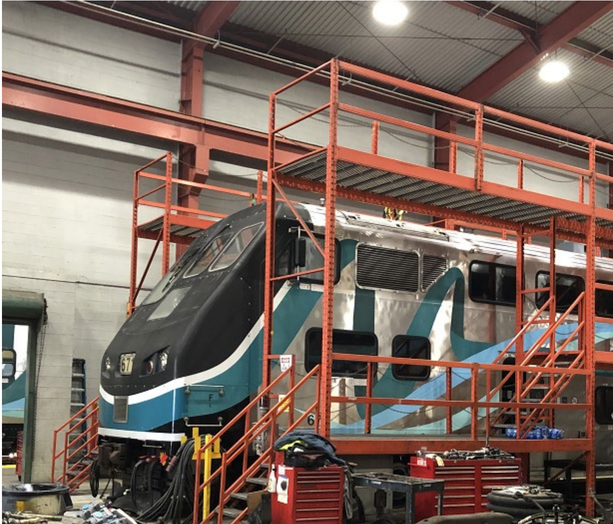
FIGURE 16-1. ULWA PLATFORM ALLOWS ACCESS TO REMOVE WINDOWS AND PERFORM ROOF WORK SUCH AS AC UNIT MAINTENANCE
