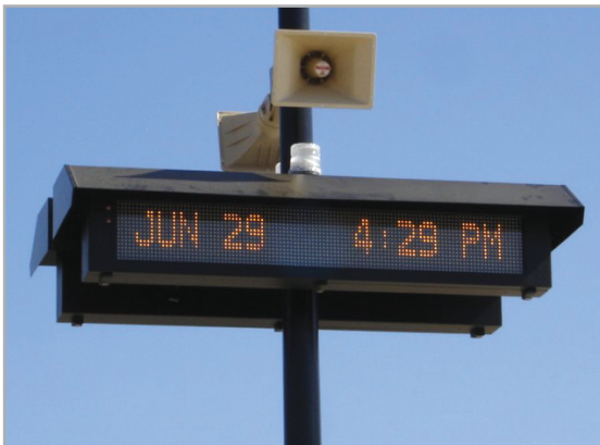
Electronic message board equipped with Public Address system technology
